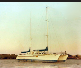
The DMB, 21m (73ft) aluminium Catamaran, cruise speed 18knots, holds 16t of seawater for live shell transportation
